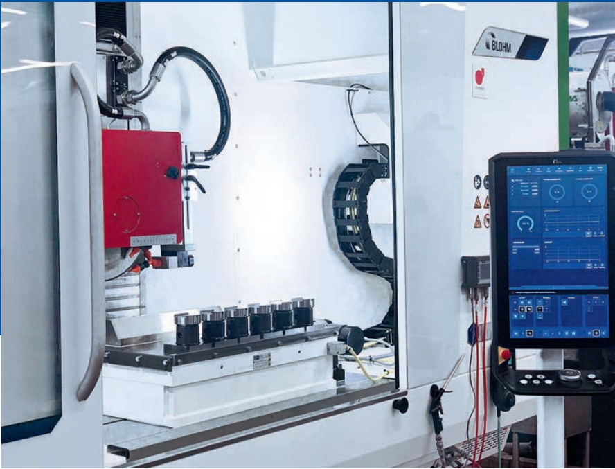
Manufacture of modular precision tool holders on the PLANOMAT XT 408 with C.O.R.E. touch display
