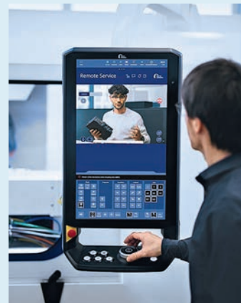
Brings the right personnel directly to the machine: In addition to chat and whiteboard functions, the C.O.R.E. panel also enables video conferencing
